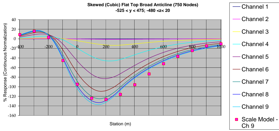
Figure 13: Comparison of the MultiLoop III and scale model data for the anticline with the cubic right limb.
